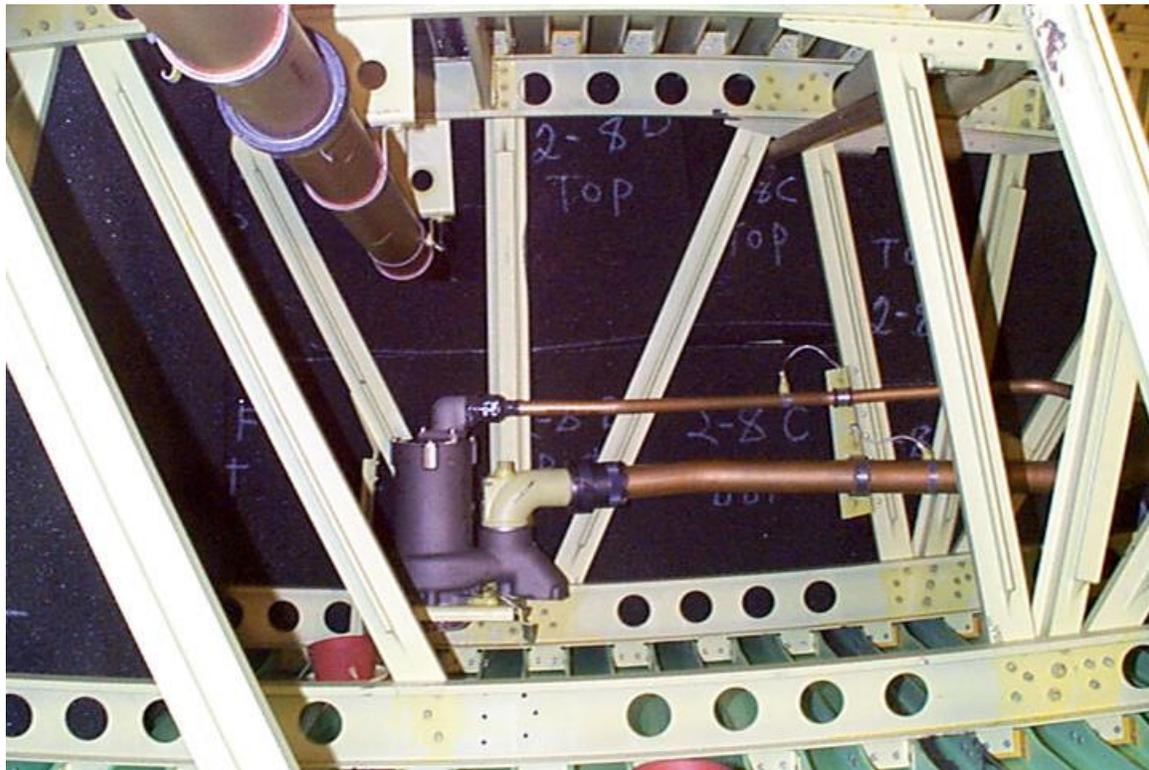
**Figure 2 - C-130 Fuel Tank with Foam Installation Ongoing
