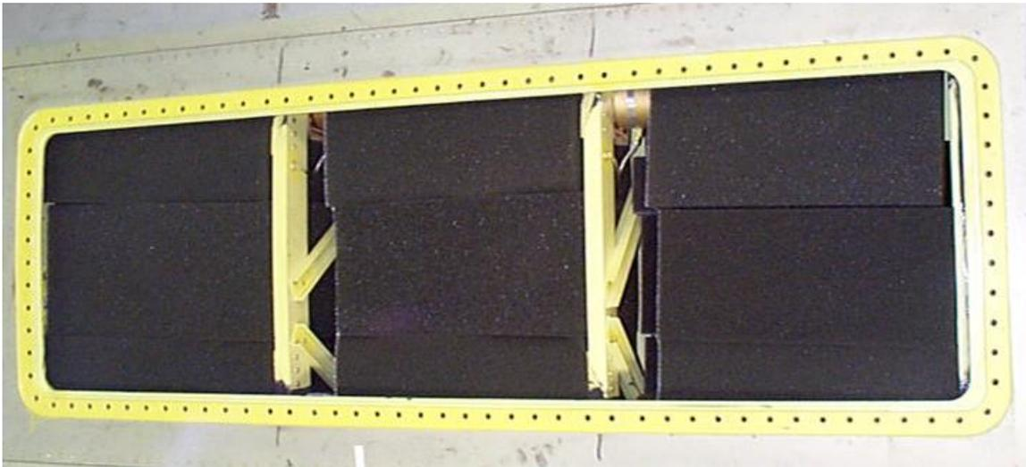
**Figure 1 - C-130 Fuel Tank with Foam Installed**
