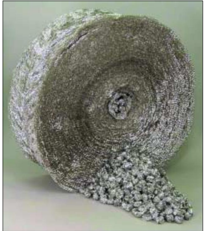
Figure 1. Two forms of expanded-metal networks. (Courtesy of Explosion Prevention Systems LLC.)
